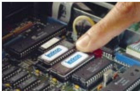
Updating your existing Model 300 is a snap – just plug in the new ROMs
