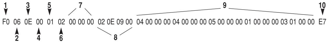
The Sample Data Message that appears above could be sent by or to the MPX 100. It could be sent by the MPX 100 in response to the Sample Query Message above, to indicate that the RtDelay1 parameter has a value of 09E2. It could also be sent to the unit to assign a value of 09E2 to the RtDelay1 parameter.
