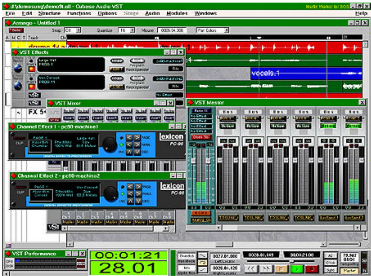
Figure 1: Main VST Screen. Both Lexicon reverb modules can be used as either Channel effects (as shown here) or as Channel inserts. Notice that the Buss Output has been set to 'PC-90 1' and 'PC-90 2' in the VST Effects window, to route Aux Sends 1 and 2 to the PC-90 hardware. The VST Master window shows the two active busses.
